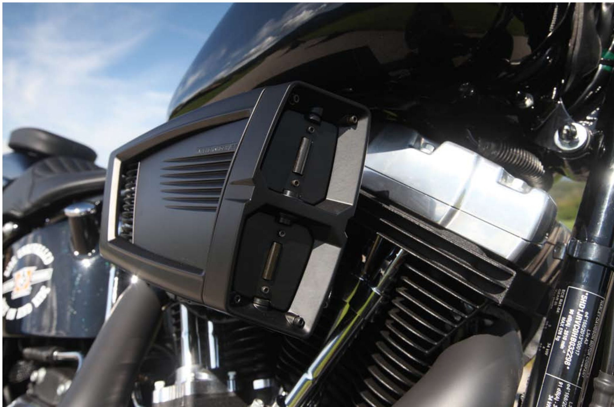
Hypercharger ES: The input impulse signals for the opening angle of the butterfly valves are taken directly from the firing sequence of the ignition coils.
