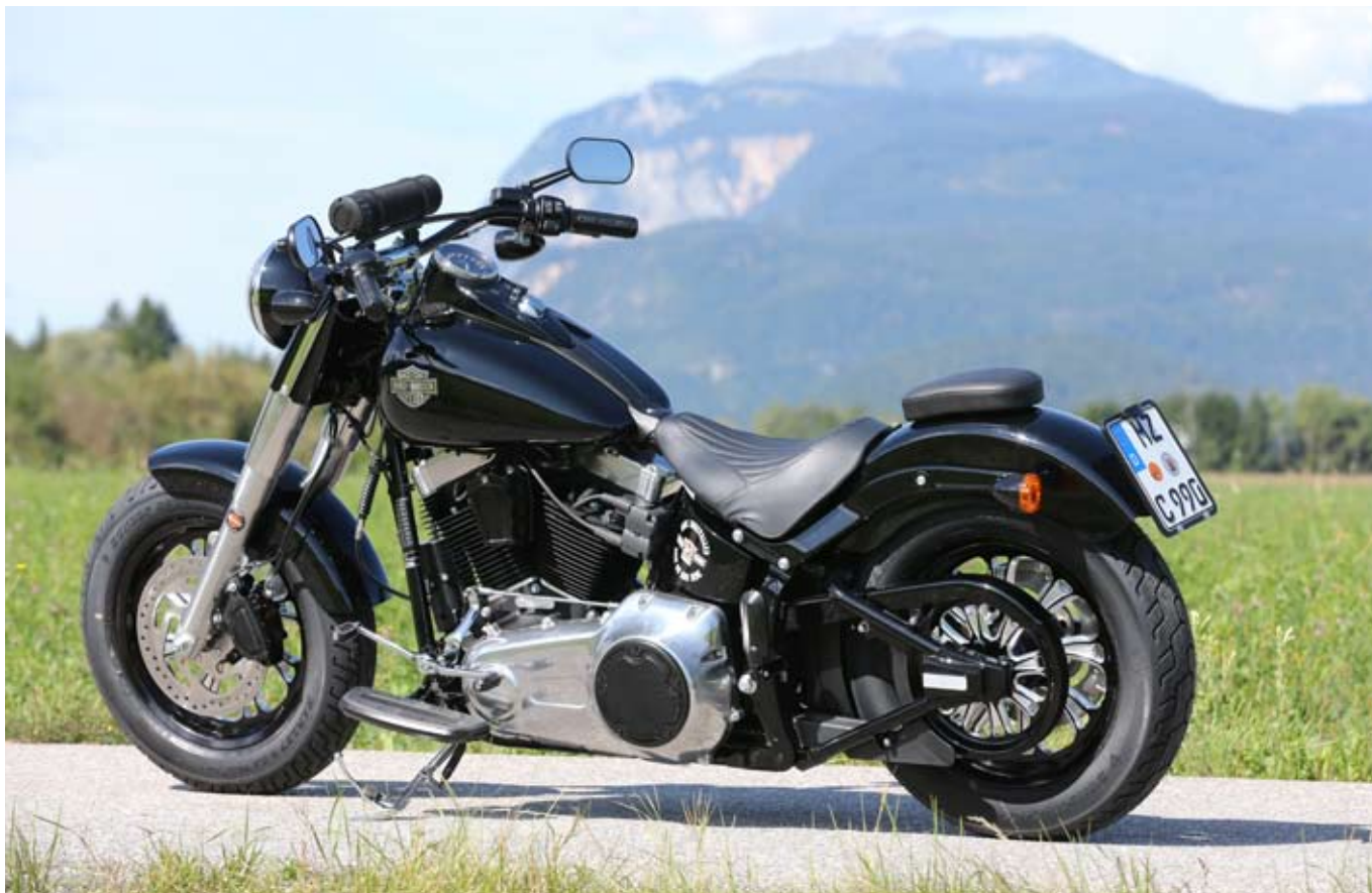
TOP: The new RevTech wheel set includes fitting belt pulley, but not yet the also available design rotors: Bobber-size is 3.5 x 16" RevTech Super Charger" Midnight Series. Frame and motor remained stock and offer a reliable power output. The seat pad is not really for long distance touring but great to have.
